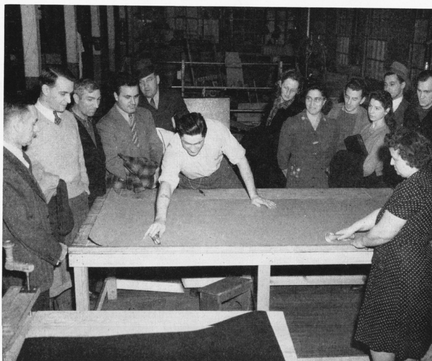
Nick Pilla, Store 7, is showing the use of his prize winning Victory Committee War Production suggestion, to employee members of the Committee. Nick devised a special scoring table with cutters for making waterproof paper bags, a production job the Store has taken on for the shipment of military parts made here.
