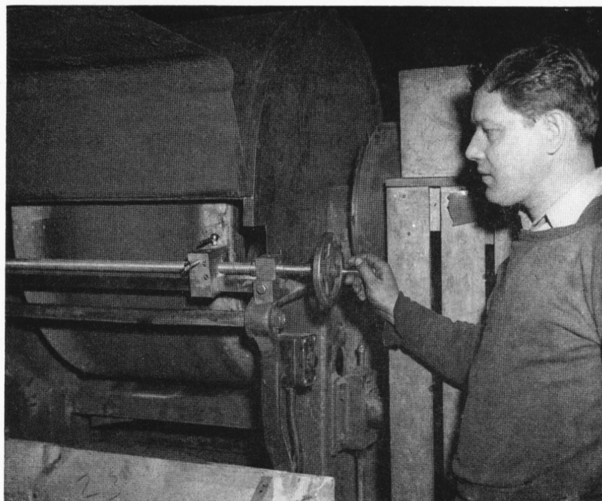
Charles Pranulis demonstrates his new idea for redressing a surface of the Weisbecker machine in the North Mill. This special mechanism, which consists of a cutting tool that is moved by screw drive across the surface of a revolving roll, is a great time and labor saver. For suggesting it Charlie took a First Prize in the November-December period.
